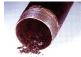
Corrosion of piping
