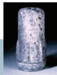
Rapid corrosion of untreated aluminium
